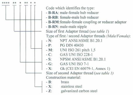
The Adaptors type **B-RM** and **B-RN** have both NPT threads or both Metric threads or coupling NPT-Metric threads.
